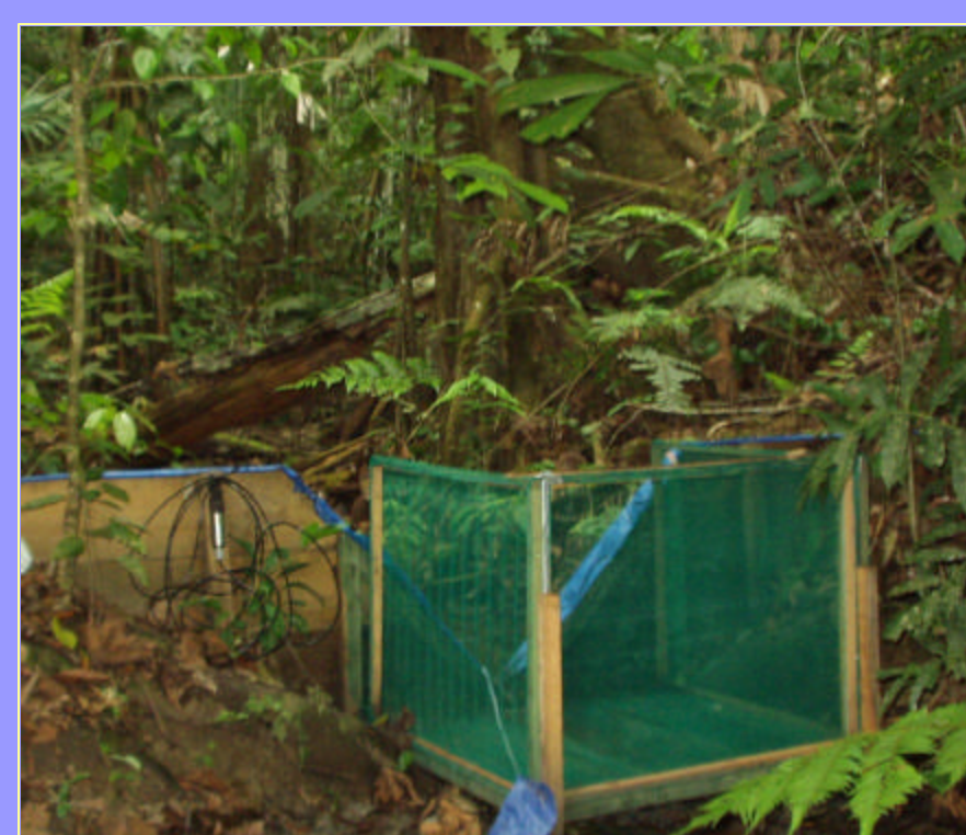
V-Notch Weir and POC trap (> 2mm)
